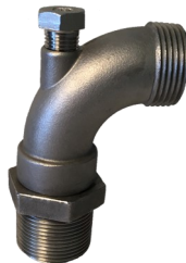
L2QCVPSWIVEL-010 304 stainless steel 1" MPT inlet 1" MGHT outlet
