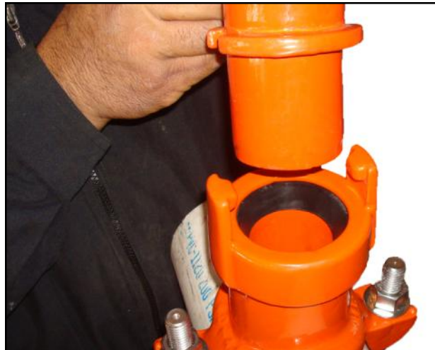
Picture of lateral valve inlet and lateral saddle bell outlet
