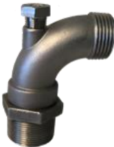
L2QCVPSWIVEL-007 304 stainless steel 1" MPT inlet 3/4" MGHT outlet
