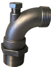
L2QCVP-SWIVEL-007 304 stainless steel 1-1/4" MPT inlet 3/4" MGHT outlet
