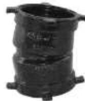
Tapered bell allows 1-21 degree pipe deflection
